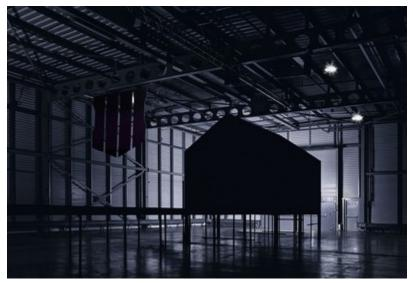
UK based Surrey Nanosystems developed Vantablack for use primarily in space applications due to its unique properties that absorbs 99.965% of natural light. The VBx2 coating, used to create the Black Ops House, was designed to reduce reflected light to such a level it becomes extremely difficult to discern any surface features on an object, making a three-dimensional object appear as a mesmerizing, two-dimensional black void.
